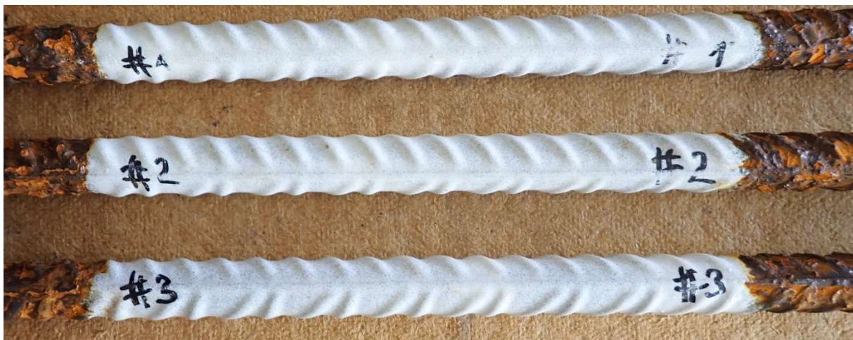
Figure 10: After 240 hours of NSS testing, the anchors show no signs of corrosion or fissuring of the coating in the area under consideration
