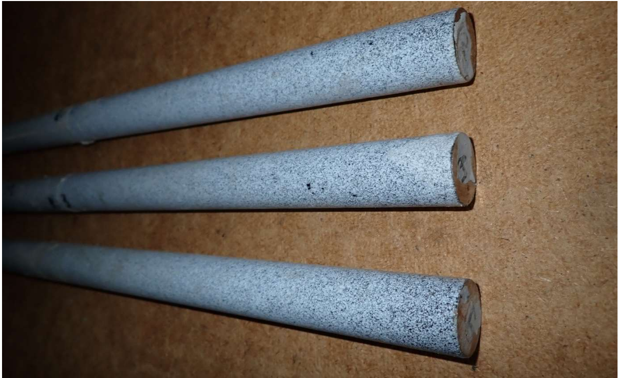
Figure 2: Surfaces of the dowels without damage of coating after the pull-out test
