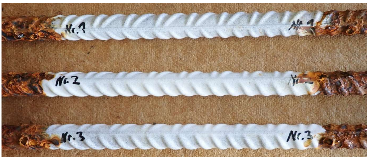
Figure 11: Opposite side surfaces of the anchors after NSS-test without signs of corrosion or fissuring in the coating
